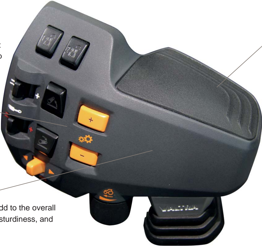
Safety usage: Area between buttons gives your thumb the possibility to rest without keeping the finger on top of the buttons. Hums around linear levers prevents error usage
